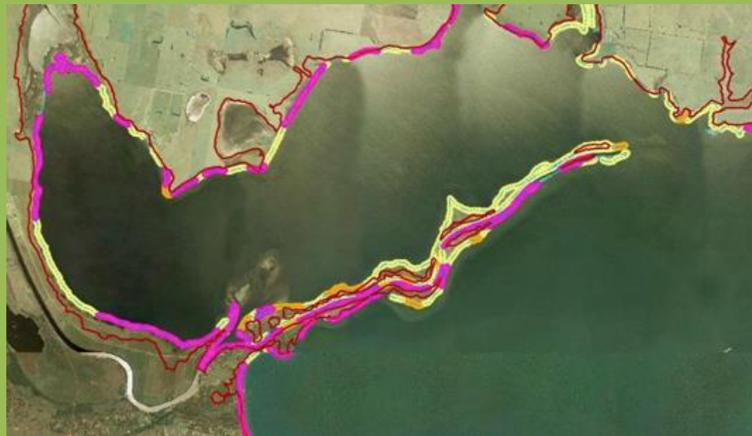
Shoreline erosion susceptibility (high shown in pink) of the areas around the silt jetties from predicted sea level rise (Arrowsmith et al. 2014).
