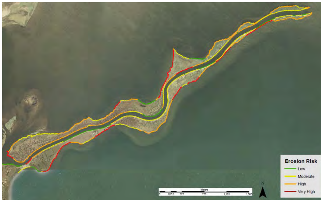
Figure 2. Erosion risk: This map shows areas identified as being at the greatest erosion risk across the site, using a combination of the information collected from the technical investigations. In essence, \text{Erosion Risk} = \text{Excess energy} \times \text{Level of resistance}
