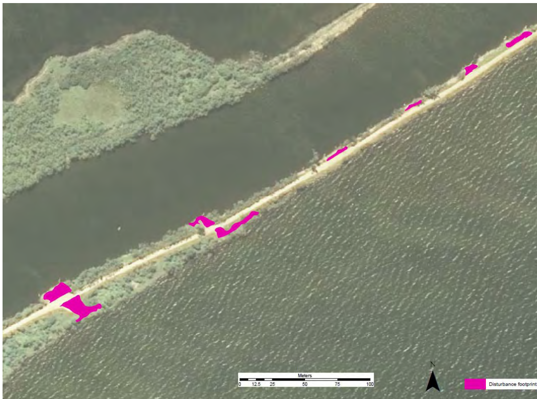
Figure 1. Site Disturbance Assessment: site visits were undertaken along the length of the silt jetties to note and map areas of disturbance. Assessments were made of road and track location, road drainage, river and lake access points. This assessment noted 57 areas of disturbance (46 informal, 11 formal), with over 4000m 2 of vegetation impacted or removed at informal access points. Issues relating to this disturbance include drainage at informal access points, drainage from the road, and inability for vegetation to establish dues to spatial constraints.
