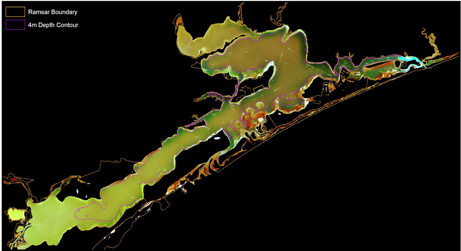
Figure 16. False colour image of the saline water region of the Gippsland Lakes Ramsar Site that seagrass was mapped in. False colour red-edge, green, blue histograms equalised shows seagrass beds as red patches (image date 24/01/2021).
