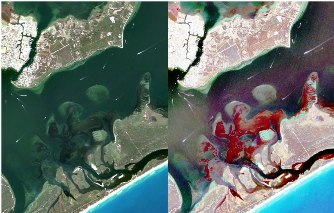
Figure 14: Normal red,blue,green (RGB) image of seagrass south of Paynesville/Raymond Island (left side) compared to a false colour image (right side; red edge sentinel band5 substituted for red). Equalising colour histograms helps visualise the seagrass beds as bright red patches from which to collect training data and to check classification outputs.
